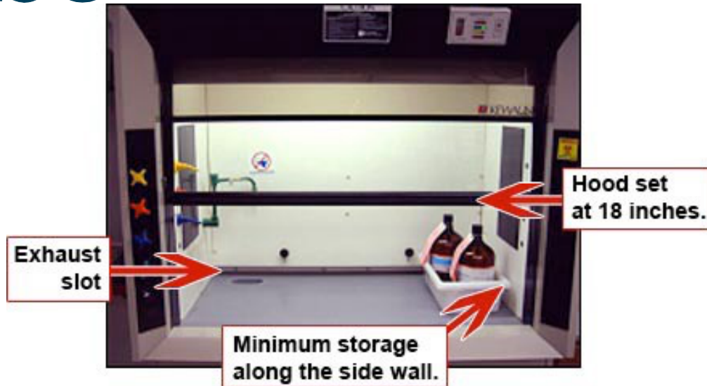
Figure 1. Properly maintained Fume Hood
