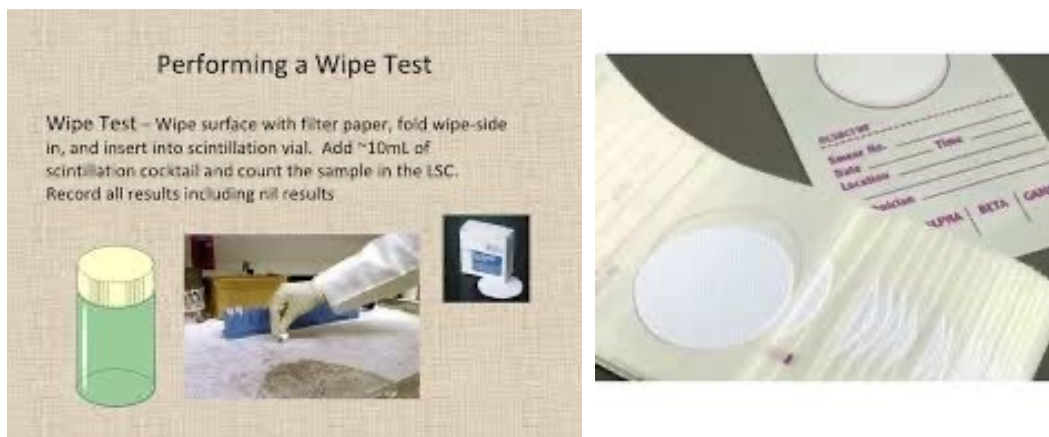
Figure 5. Wipe Test Procedure and Wipe Test Plate
